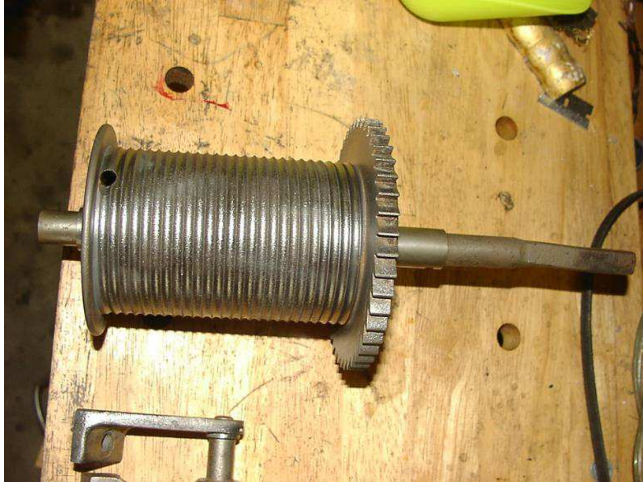
Drum chemically cleaned and wire brushed
