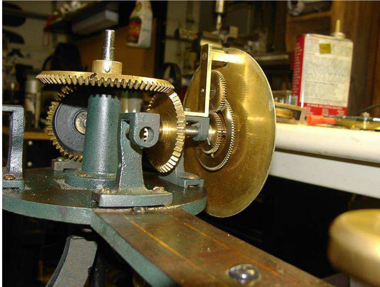
Motion work and drive (bevel) gear, backside of dial also made for this clock
