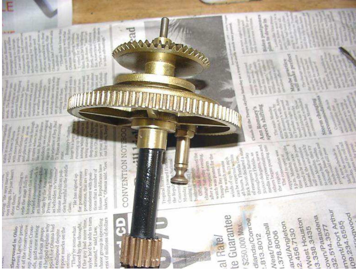
Center shaft assembly after cleaning and paint
