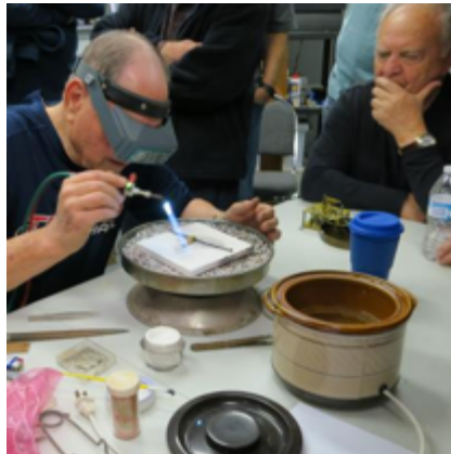
Val Link shows how to fill a worn pivot hole using silver solder
