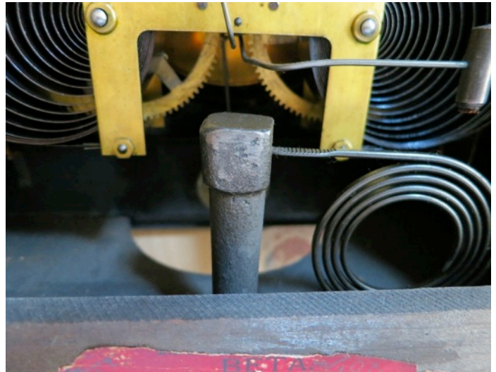
Figure 11. Rear view inside case showing hole in base for pendulum bob access.
