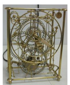
However, this is merely an illusion. The little men actually do no work at all. The clock is powered by a synchronous motor that turns the first wheel in the time train, and the men follow the power provided to the time train."
