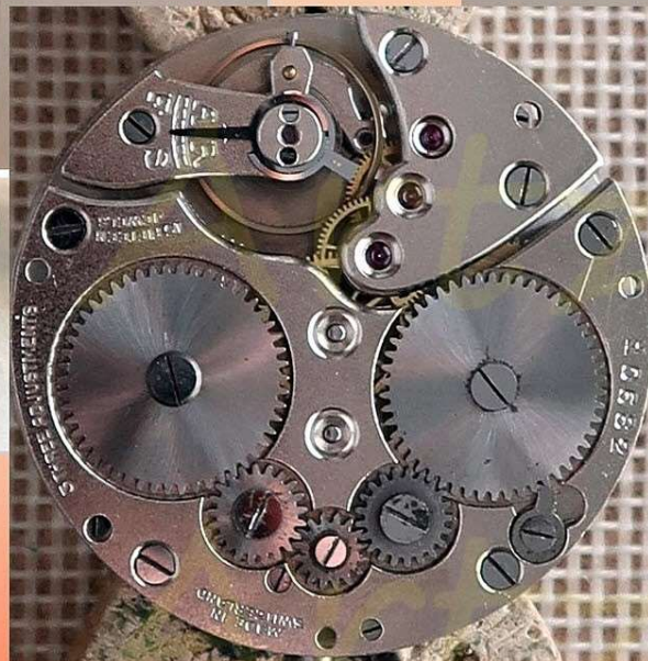
LANCEL (French) table lighter with 8 day, 15J, Adj 3 pos, Swiss clock. Circa. 1930.
